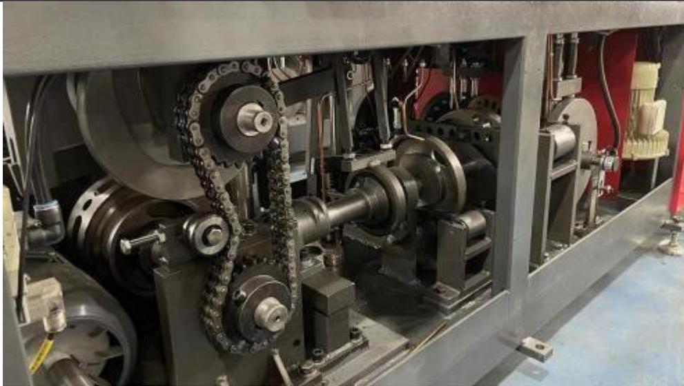
1. The whole **Open Cam Paper Cup Machine** adopts automatic oil lubrication system( oil circulation system is including oil motor,filter, copper pipe )which makes all gear moving parts working at high speed much more smoothly and greatly Improve the service life of spare parts.
